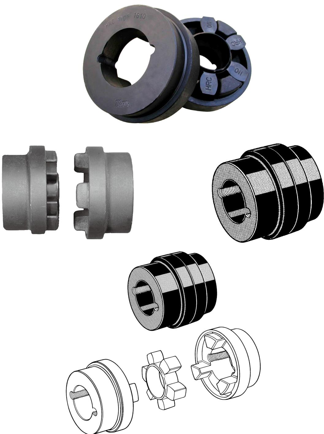
These semi-elastomeric couplings are designed for general purpose applications and permit quick and easy assembly by means of Taper bush. Outside diameters are fully machined to allow alignment by simple straight edge methods. Shaft connection is "fail safe" due to interacting jaw design.
