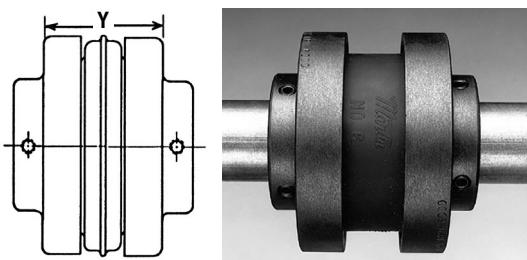
**Step 5.** Slide loose flange on the shaft until the sleeve has seated completely in teeth of both flanges. Refer to "Y" dimension although not a critical dimension. Secure the flange to shaft and torque set screws and cap screws to correct torque values.
