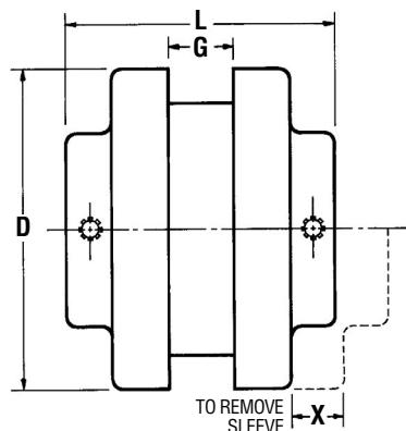
Type S flexible coupling flanges are bored to size to fit on any standard shaft. They are produced from high strength cast iron. Units are easy to install and remove and are stocked in a wide range of bore sizes as shown on the next page.
