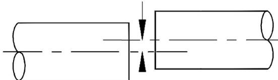
**PARALLEL MISALIGNMENT** - Shafts are in line angularly and parallel to each other, but are off-set.
